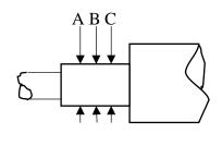
A. SHAFT RADIAL RUNOUT \_\_\_\_\_
